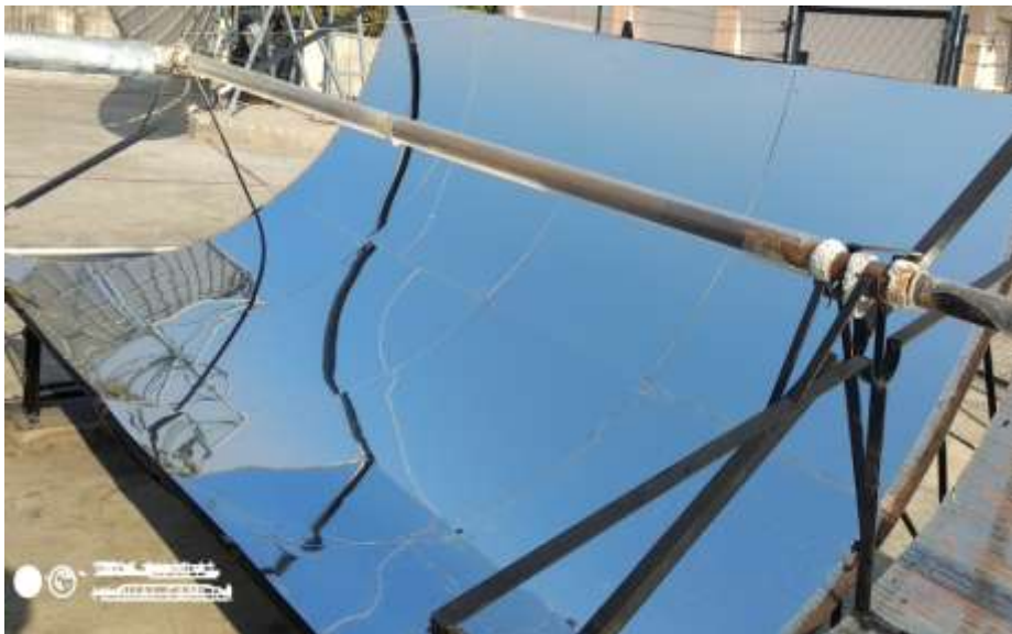
Fig.3. CPC with anodized aluminum (MIRO-SUN) as reflector material (Image)
