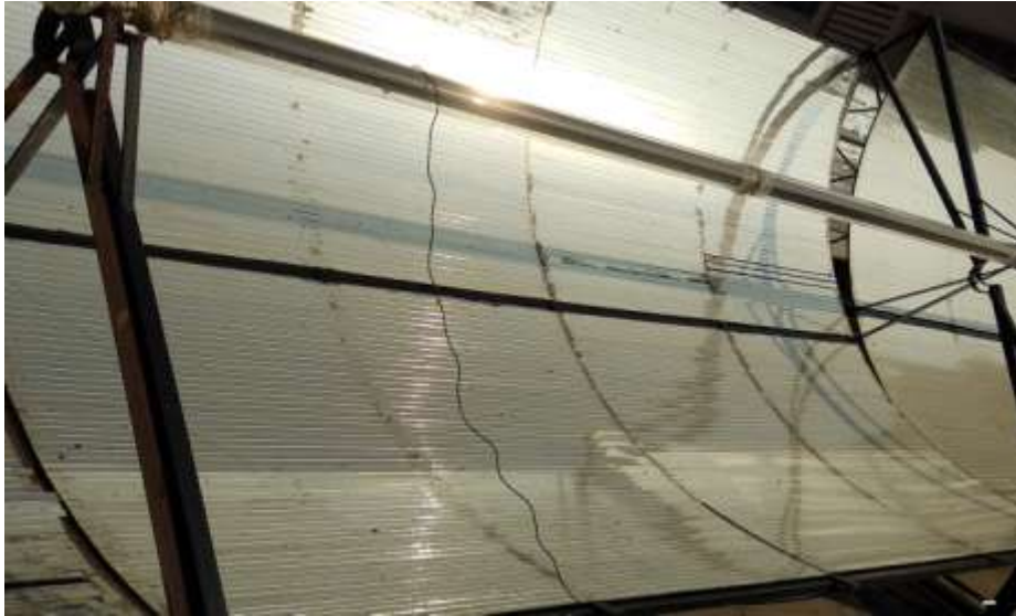
Fig.2. CPC with mirror as reflector material (Image)
